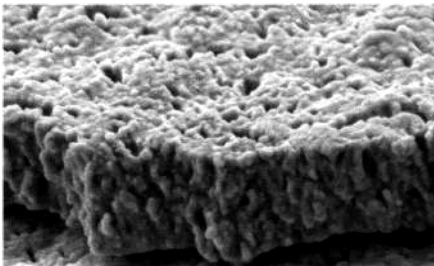
*Figure 5. SEM micrograph of porous SiO<sub>x</sub> flake. The estimated pore density is  $3 \cdot 10^9 \text{ gcm}^{-2}$ . The root mean square (RMS) roughness is between and 3 and 20 nm. Pore sizes according to BET measurements are between 2 and 5 nm with a maximum at 3 nm.*
