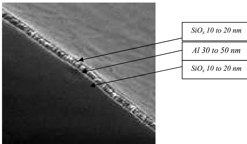
Figure 2. SEM micrograph of SiO<sub>x</sub>/Al/SiO<sub>x</sub> sandwich. Thickness of: SiO<sub>x</sub> 10 to 20 nm, Al 30 to 50 nm, SiO<sub>x</sub> 10 to 20 nm
