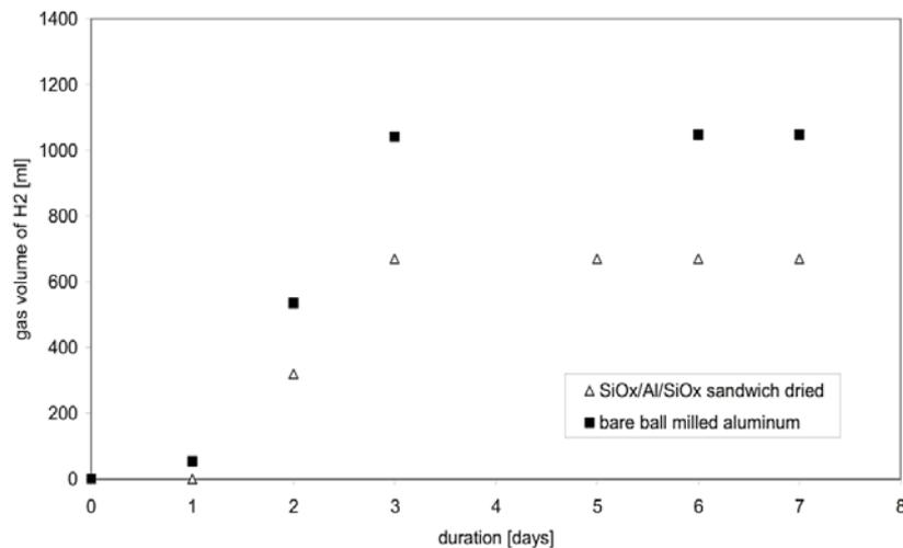
Figure 4. Amount of generated hydrogen in protected ( $\Delta$ ) an unprotected Al ( $\blacksquare$ ) by aqueous Corrosion medium (2% Akropal N100). The gas volume is standardized on the Al content.
