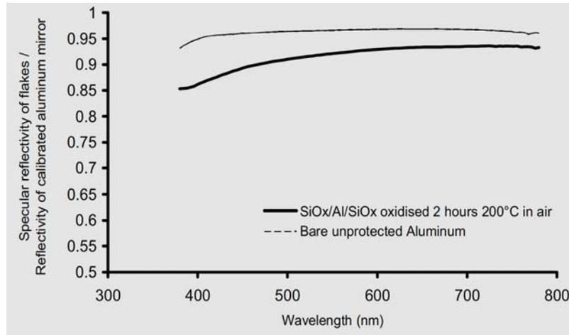
Figure 3. Reflectivity of bare aluminum flakes (--) and heated SiO<sub>x</sub> protected Al flakes (—).
