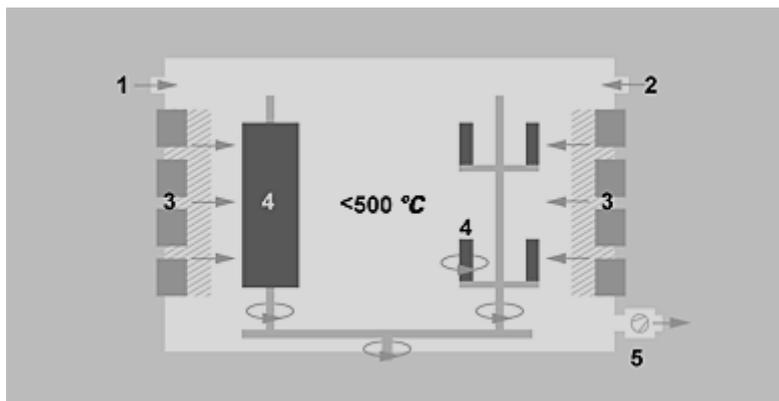
Figure1. The schematic device used in the manufacture of sandwich layers; 1. Argon; 2. Reactive gas; 3. Arc sources (coating material and backing plate); 4. Components; 5. Vacuum pump
