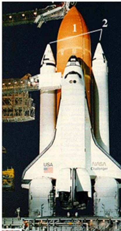
Figure 1. Challenger, the launching day. 1. External tank. 2. Solid rocket boosters [3].
