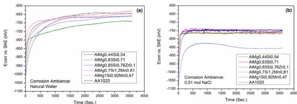
Fig. 2. Open circuit potential vs. time graphs of tested 6000 samples in (a) natural water and (b) 0.51 mol NaCl solutions, open to air at room temperature
