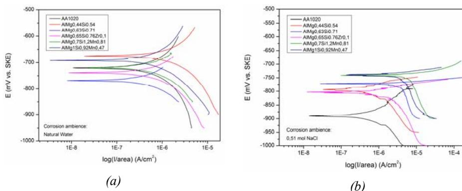
Fig. 4. Potentiodynamic polarization diagrams for investigated 6000 alloys' samples immersed in (a) natural water and (b) 0.51 mol NaCl solutions, at room temperature.
