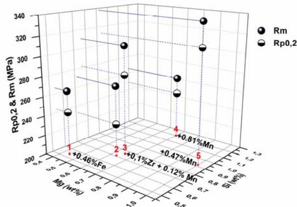
Fig. 1. Tensile properties of investigated 6000 alloys after the artificial ageing, as a function of the content of alloying elements.
