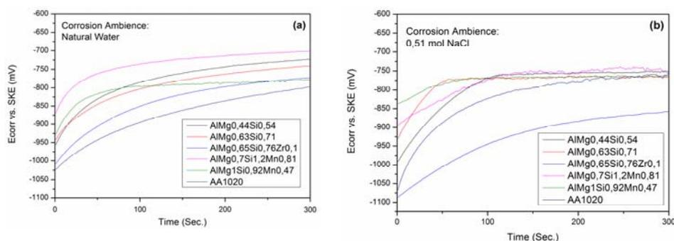
Fig. 3. Open circuit potential vs. time graphs of tested 6000 samples in (a) natural water and (b) 0.51 mol NaCl solutions, open to air at room temperature during the first 300 seconds
