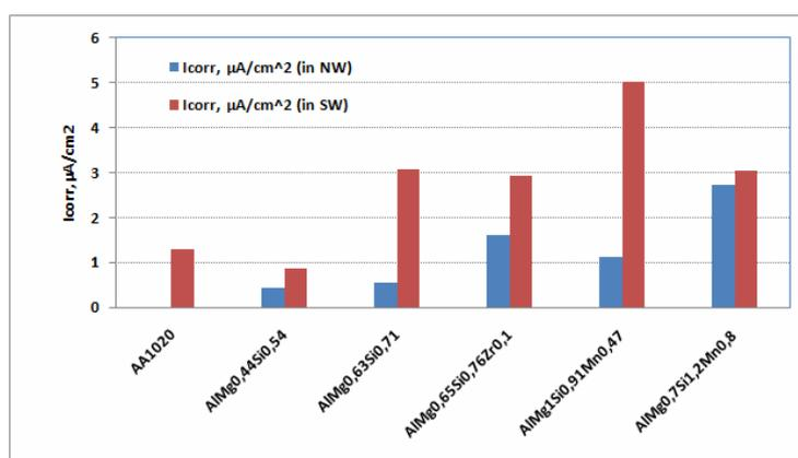
Fig. 5.  $I_{corr}$  of artificially aged samples of tested alloys under potentiodynamic conditions in both corrosion ambiances.
