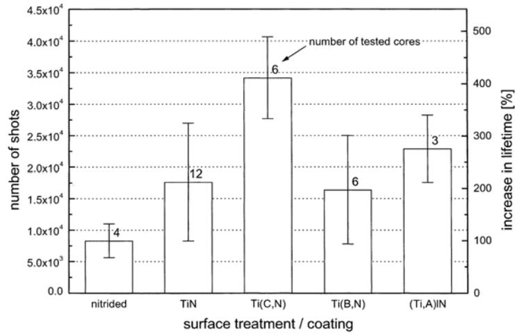
Figure 1. Number of shots achieved in aluminum pressure dies casting for cores of oil pump housing for nitriding and different PECVD coatings. The end of the lifetime is determined by insufficient surface quality of the casting.
