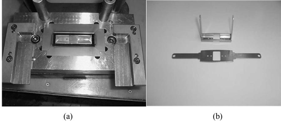
Figure 4. PECVD Ti(C,N) coated forming tool (AISI A11 cold- worked steel) and parts produced using this tool.
