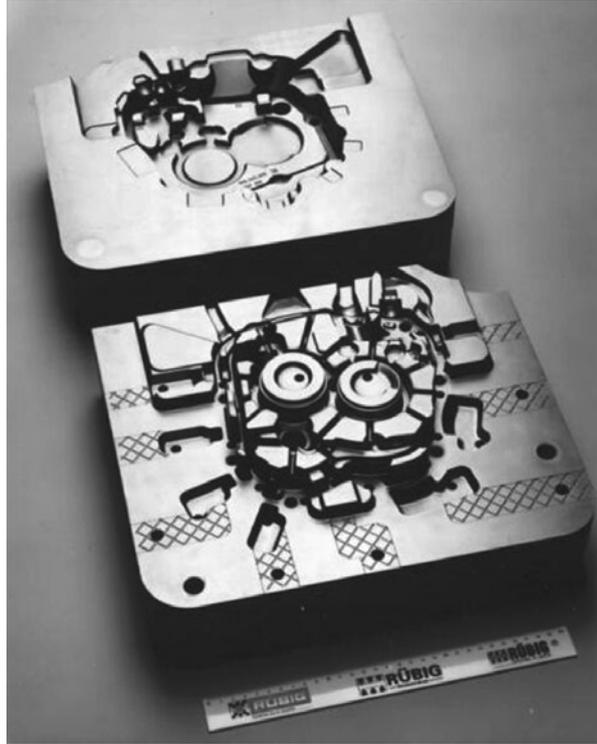
Figure 2. PECVD Ti(C,N) coated die (AISI H13 hot worked steel) for aluminum pressure die casting of an oil pump housing.
