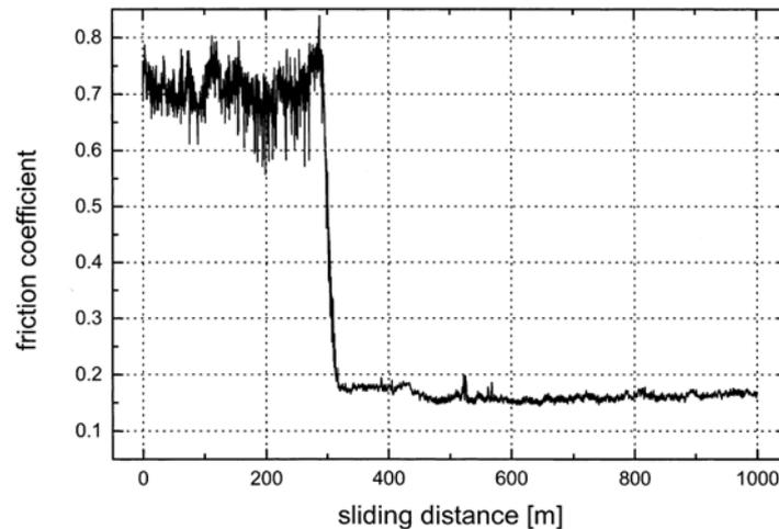
Figure 5. Dependence of the friction coefficient of an unalloyed steel ball sliding against a PACVD TiN coated disc on the sliding distance (normal load, 2 N; sliding speed 10 cm/s; relative humidity, 35%).
