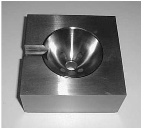
*Figure 3. PECVD Ti(C,N) coated injection mold (AISI H11 hot work steel) for an automotive headlamp.*
