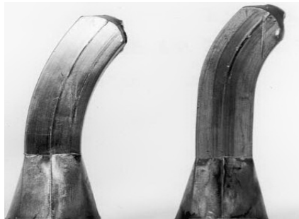
Fig. 1. Deviation of product after exiting the die [10]
