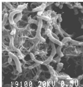
Fig. 3. Biofilm formed by sulfate-reducing bacteria on the surface of mild steel, visualized using SEM [6].
