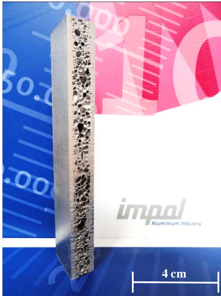
Fig. 6. The cross-section of the prototype core-foamed panel made from ARB precursor with dolomite particles as the foaming agent.
