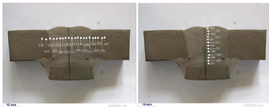
Figure 4 Hardness measurements of weld deposits along horizontal line (a) and vertical line (b) - welding with MPW1, AW condition
