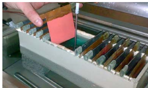
Fig.2. Copper deposited on the cathode
