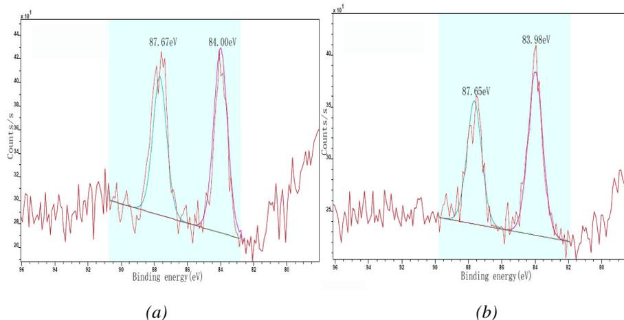
Fig. 3. XPS analysis for Au nanoparticles (a) for copper immersed in rabbit IgG solution for 10min; (b) for copper implanted in rabbit uterus for 10min
