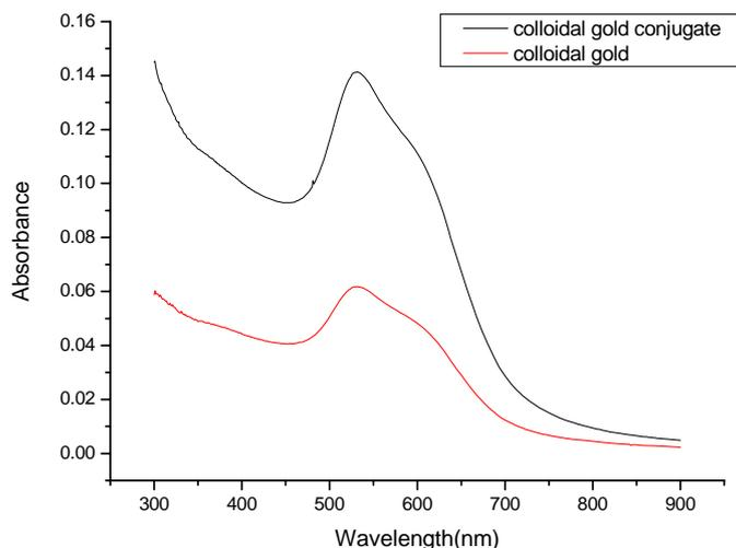
Fig.1. UV-vis spectra of unmodified gold nanoparticles and nanogold labeled goat-anti-rabbit IgG.
