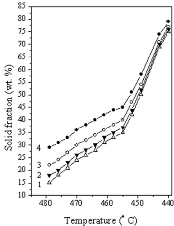
Figure 2. Solid fraction dependence on temperature during isothermal solidification. 1) SSM of ZA27 alloy; 2, 3, 4) SSMs of composites with 3, 8 and 16 wt. %  $Al_2O_3$ , (250  $\mu m$  particle size), respectively.
