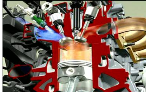
Picture 2: Cross section of cylinder head
