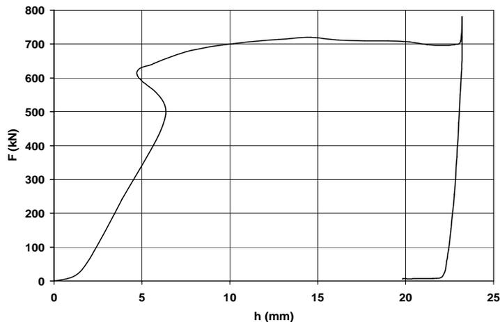
Fig. 4:  $F(h)$  diagram – Experimental phase II – dynamic investigations –
