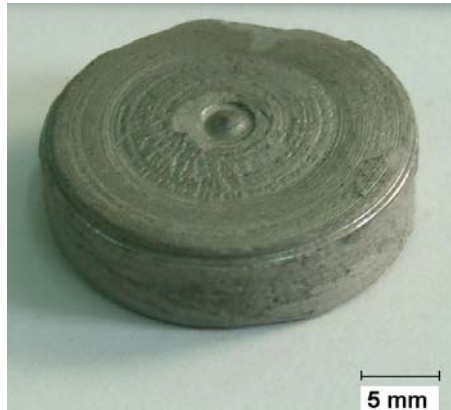
Fig. 3: Tungsten specimen obtained through underwater explosive compaction method
