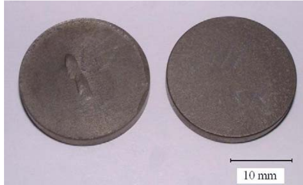
Fig. 2: Tungsten specimens obtained through Powder metallurgy technique
