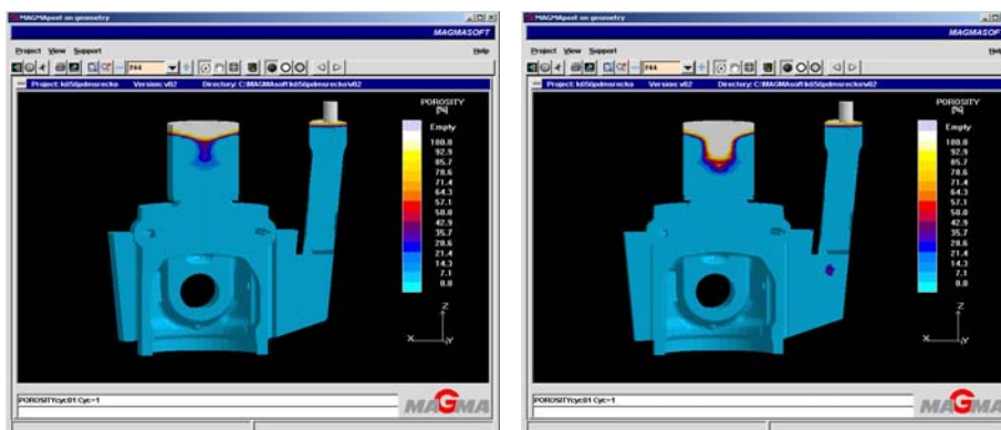
Slika 11. – "POROSITY" analiza odlivka klipa [1] Figure 11. – "POROSITY" analysis of piston casting [1]
