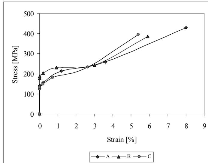
Fig. 5. Stress-strain curves of quenched specimens of the alloy A, B and C
