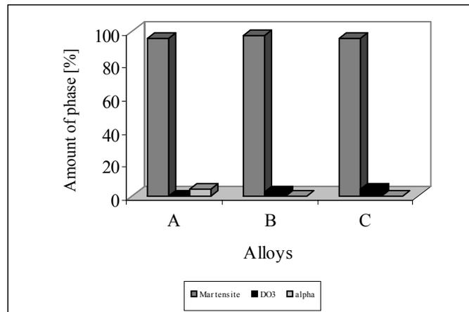
Fig. 4. The amount of various phases in quenched specimens of the alloy A, B and C
