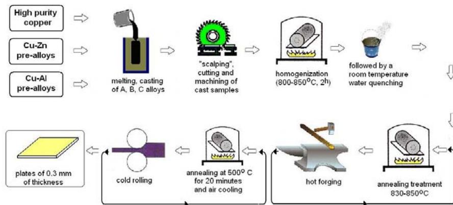
Fig. 1. Production procedure and thermomechanical processing of Cu-Zn-Al shape memory alloys
