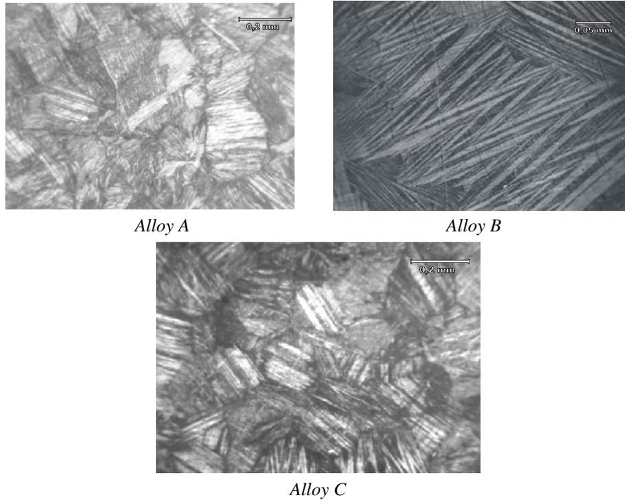
Fig. 2. Optical microstructures of quenched specimens
