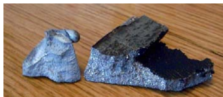
Sl.3.8. Makrostruktura ležaja: navareni (manji) i naliveni (veci) uzorak. Fig.3.8. Macrostructure of bearings produced by: weld cladding (smaller) and cast cladding (bigger) specimen.
