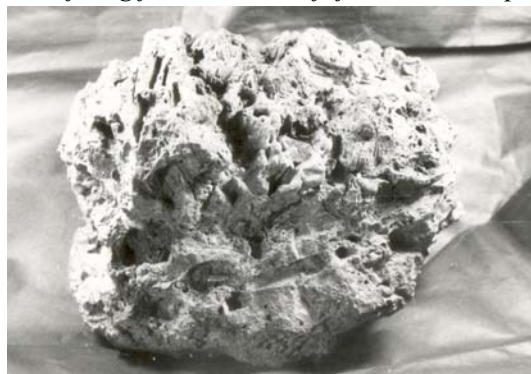
Fig. 11 – Slag from small shaft furnace, site Spišské Tomášovce
