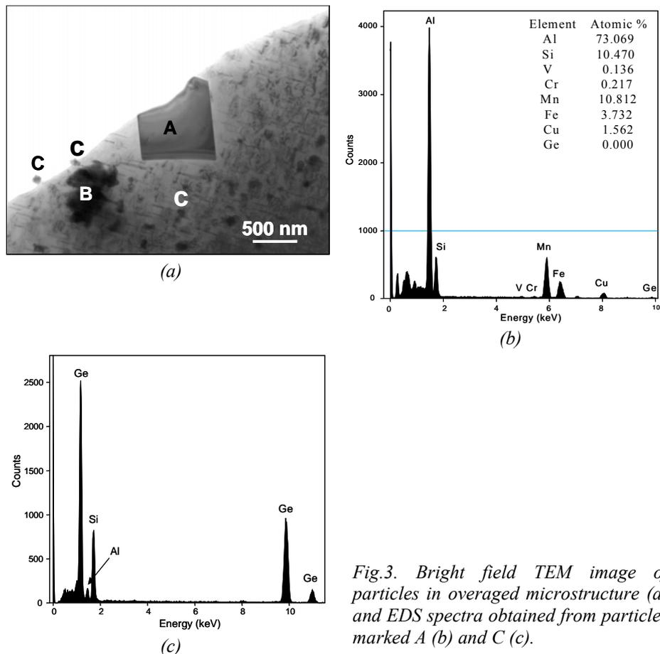
Fig.3. Bright field TEM image of particles in overaged microstructure (a) and EDS spectra obtained from particles marked A (b) and C (c).
