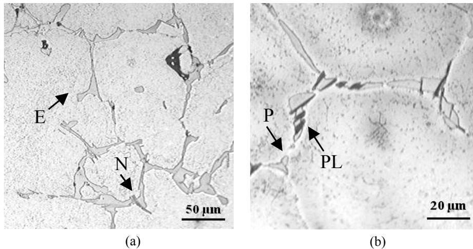
Fig.1. Optical micrographs showing as-cast microstructure of modified 2219 alloy.
