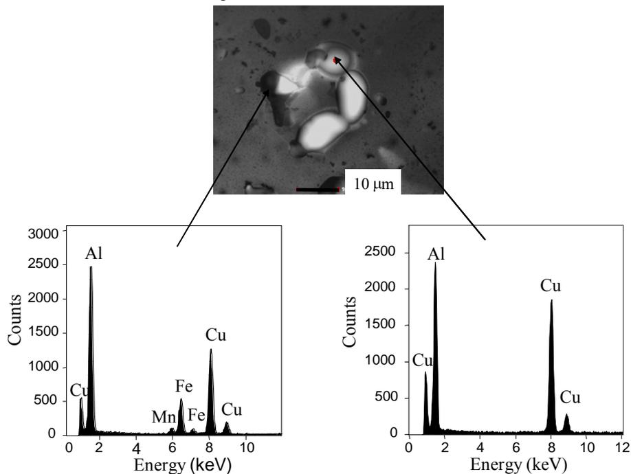
Fig.2. TEM micrograph of particles in overaged microstructure with corresponding EDS spectra.
