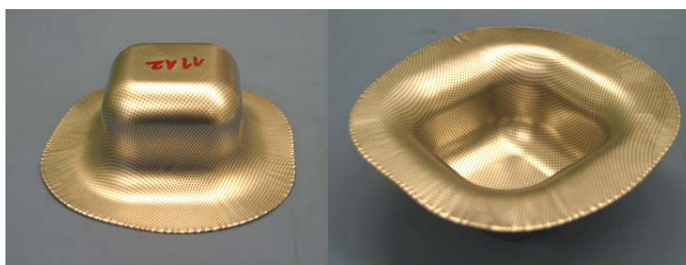
Fig. 7. Cup with layers of austenitic steel (1.4404) and a PP/PE-foil core
