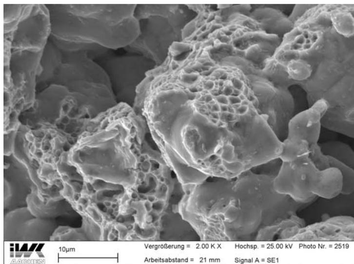
*Figure 1 - Fracture surface from the final fracture of pulsating fatigue specimens of the material Distaloy AE+0,5 %C+0,03 %B*
