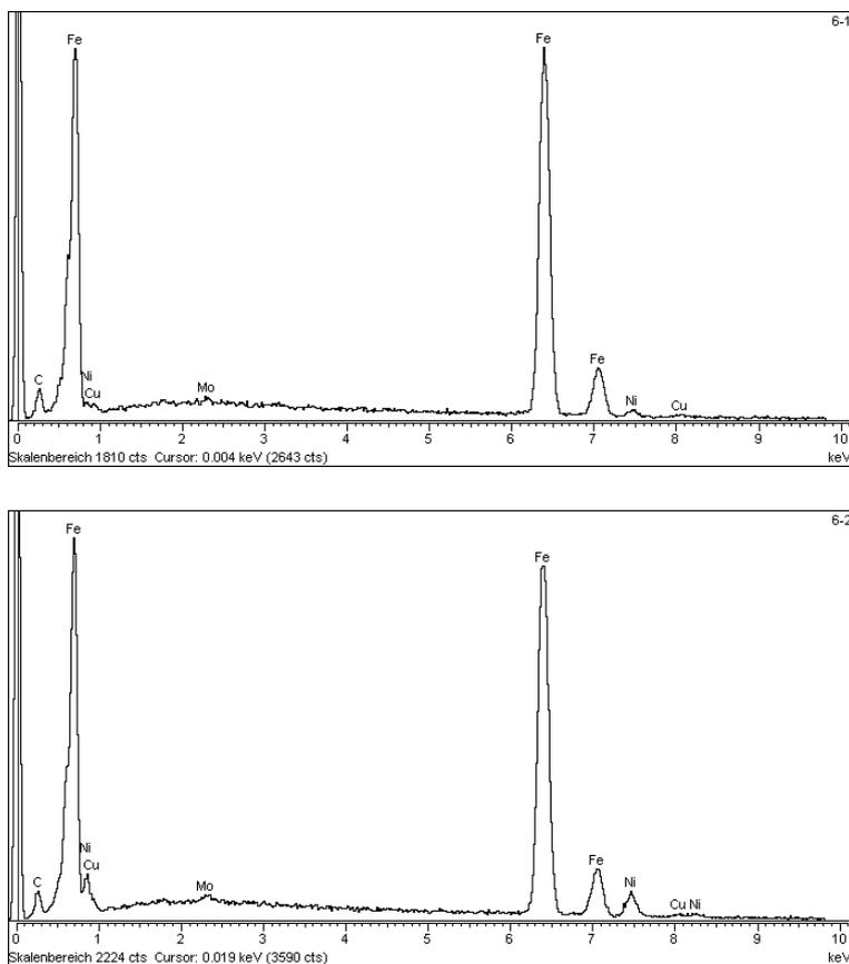
Figure 4 - Distribution of elements in different points sintered of the material Distaloy AE+0,5%C+0,06 % B shown in a fig. 3
