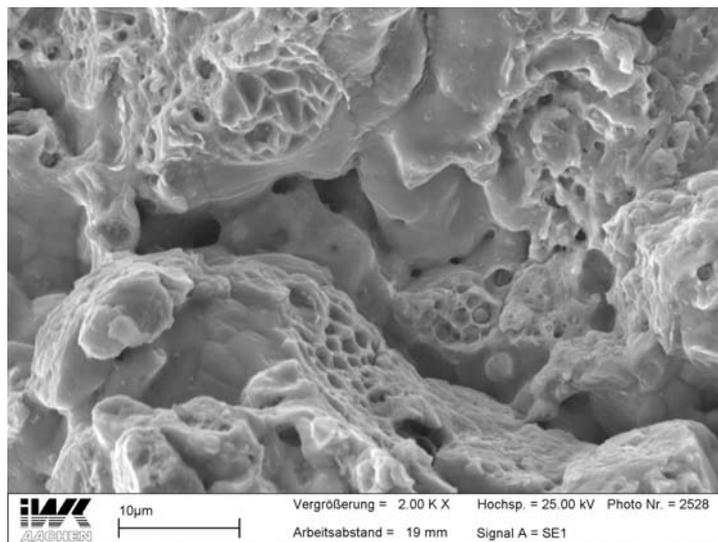
*Figure 2 - Fracture surface from the final fracture of pulsating fatigue specimens of the material Distaloy AE+0,5%C+0,06 %B*
