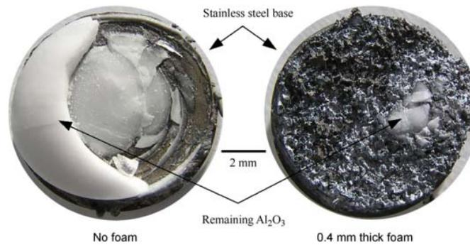
Fig. 4. Fracture surfaces of joints without and with metallic foam following thermal cycling between 300 and 800°C in air [27].
