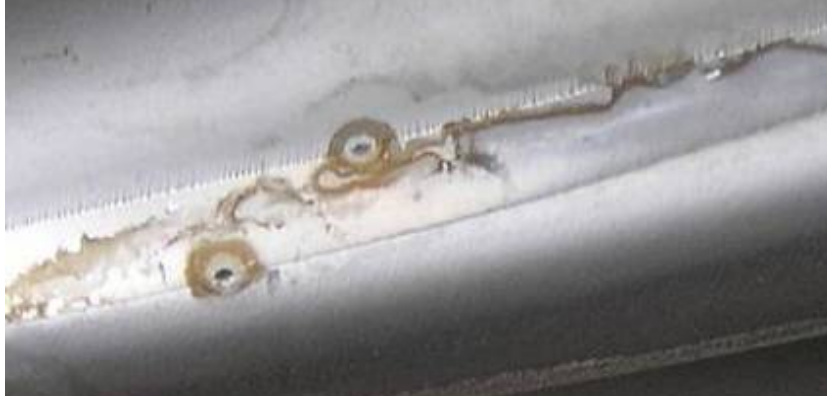
Figure 9. Surface failure of rotor coated with WC. Friction cuttings and initiation of formation of pits into the base metal due to coating thinning.
