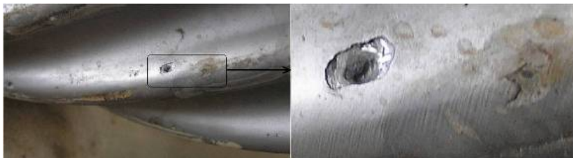
Figure 10. Surface failures of rotor coated with WC. Friction cuttings and the beginning of hole penetration into the base metal due to coating thinning. The figure on the right is enlarged detail of the left figure.
