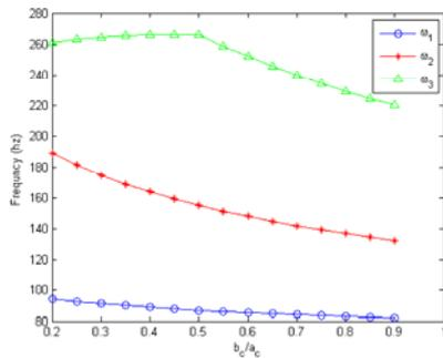
Fig. 5a Variation of natural frequencies versus ( $b_c/a_c$ ) in the composite lattice plate (a) first three natural frequencies
