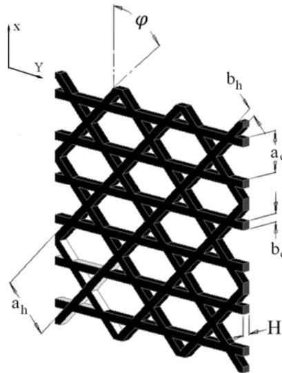
Fig 1. Geometrical parameters of a composite lattice plate
