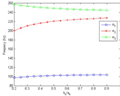
Fig. 6a Variation of natural frequencies versus  $(b_l/a_l)$  in the composite lattice plate (a) first three natural frequencies
