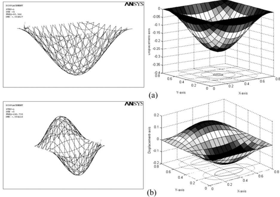
Fig. 3 The three-dimensional view to first and second mode shapes of vertical displacement ( $W$ ) respectively: (a) and (b), in the composite lattice plate
