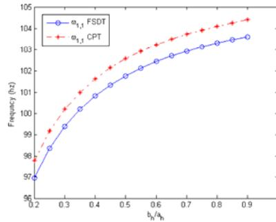
Fig. 6b Variation of natural frequencies versus  $(b_l/a_l)$  in the composite lattice plate (b) discrepancy between CPT and the present method
