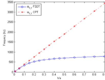
Fig. 4b Variation of natural frequencies versus ( $h/a$ ) in the composite lattice plate (b) discrepancy between CPT and the present method
