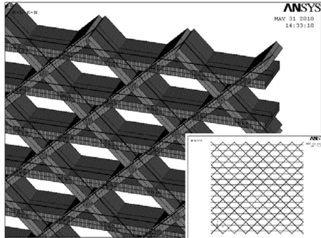
Fig. 2 The mesh generated using ANSYS package for the composite lattice plate (Example 2)
