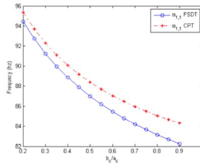
Fig. 5b Variation of natural frequencies versus ( $b_c/a_c$ ) in the composite lattice plate (b) discrepancy between CPT and the present method
