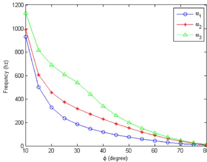
Fig. 7 Variation of natural frequencies versus  $\phi$  in the composite lattice plate
