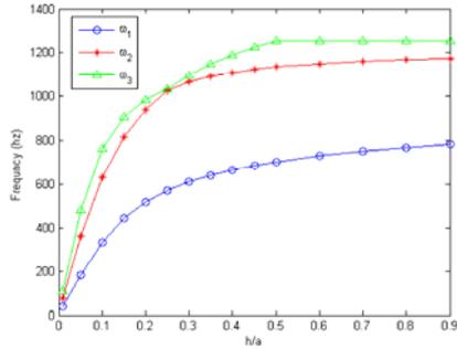
Fig. 4a Variation of natural frequencies versus ( $h/a$ ) in the composite lattice plate (a) first three natural frequencies
